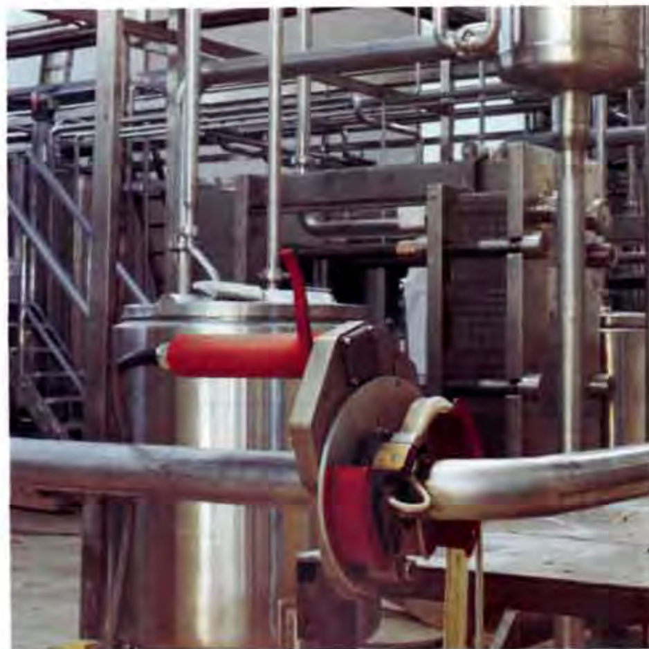
High grade High grade steel tubes are welded in a milkprocessing plant with "MU" pipewelding pliers.
